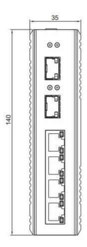
Din-rail mounting (unit: mm)
