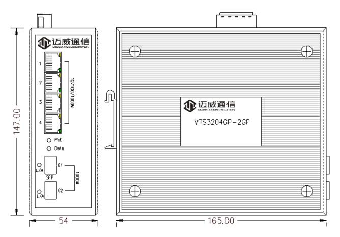
Din-rail mounting (Unit: mm)
