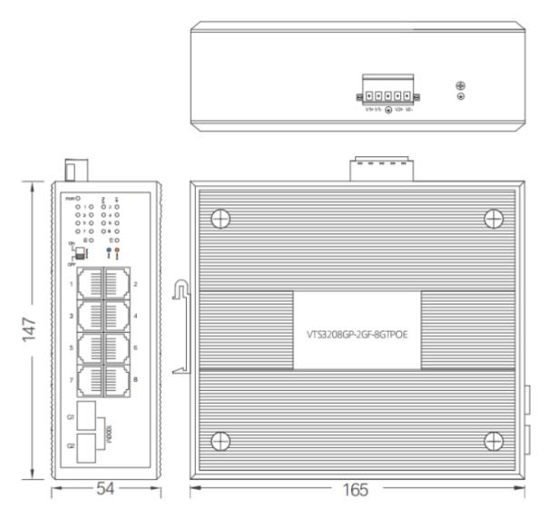
Din-rail mounting (Unit: mm)
