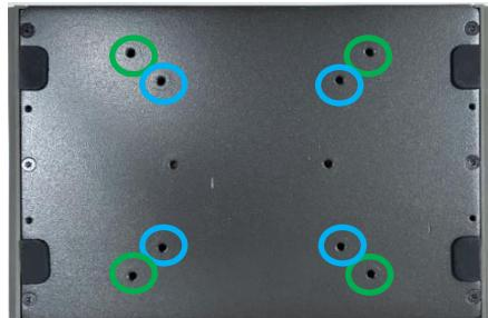
Step 1. Align the stand with the screw holes on the system, then secure it in place by tightening the corresponding number of screws as shown below. (Please note the VESA mounting holes deep 3 mm at the back of the terminal are provided with 4 x M4-type blind fasteners to fix the VESA mounting plate. A different screw length (L) should be selected.)
