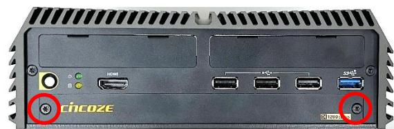
Step 2. Loosen the screw on the HDD bracket.
