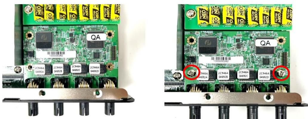
Step 5. Attach the assembled M12 I/O bracket on to the system, and fasten the hex nuts to fix it.
