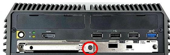
Step 7. Fasten the 2 screws on the front panel.
