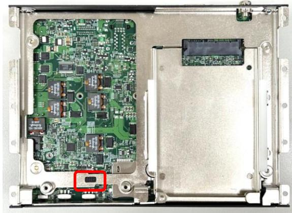
Step 2. Insert the connector of IGN module to the female connector on system motherboard.
