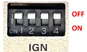
Default setting of Pin1 to Pin4 is OFF/OFF/OFF/OFF.
