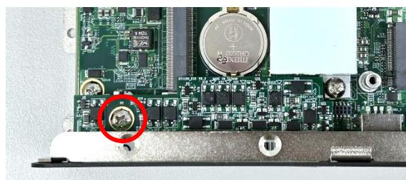
Step 5. Attach the I/O bracket on to the system, and fasten the two screws to fix it.
