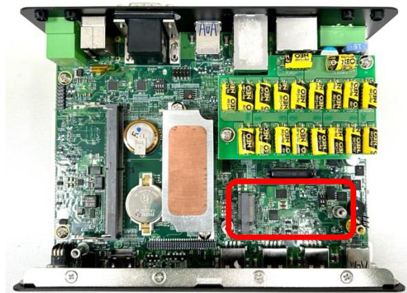
Step 2. Insert the M.2 Key B module at a 45-degree angle and insert it to the slot until the gold-pated connector of module contacted firmly with the slot.
