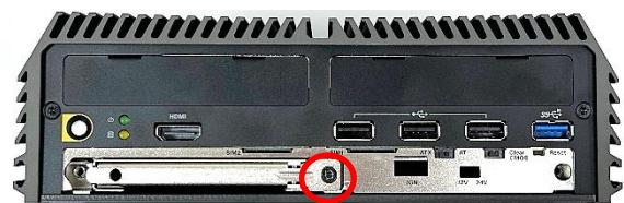
Step 3. Pull out the HDD bracket.
